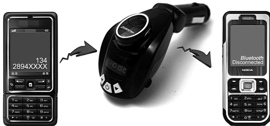
The bluetooth connection on one of the mobile has been disconnected when the other one is having a call.
